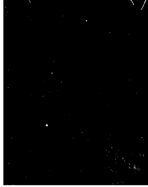
Figure 5.9.11: Mask file. Outlier pixels have a value of 0 (white) and others 1 (black). Any outlier pixels will be masked out by mutipling the mask file to images of concern.
