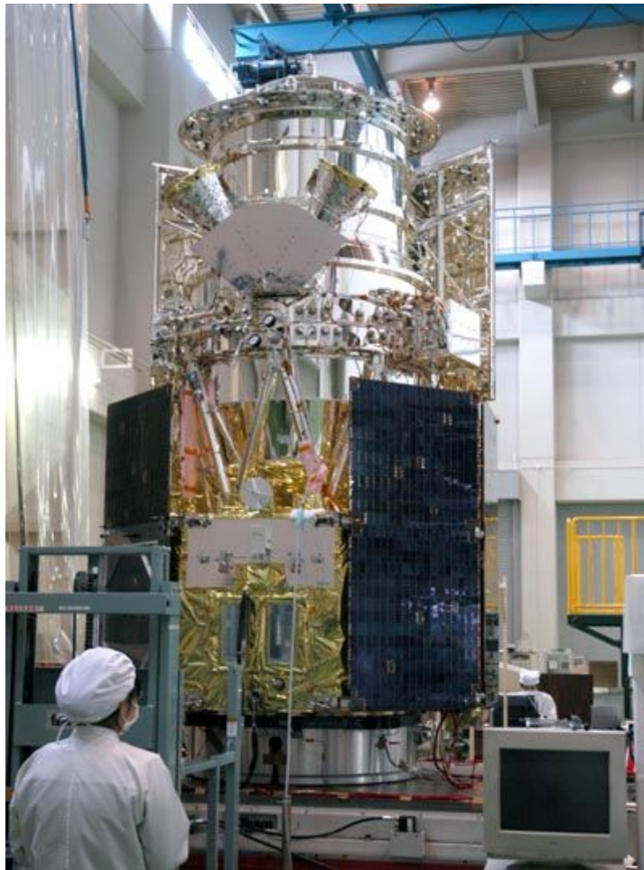
Figure 1.1.1: ASTRO-F on the vibration test bench (May, 2005).
